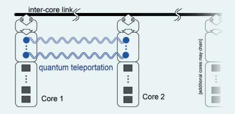
Recent work by H Jnane et al proposes a multicore architecture as a promising architecture. Multiple quantum cores are connected by an inter-core, quantum communication link, making the architecture well-suited to perform the derangement-circuit error mitigation.
