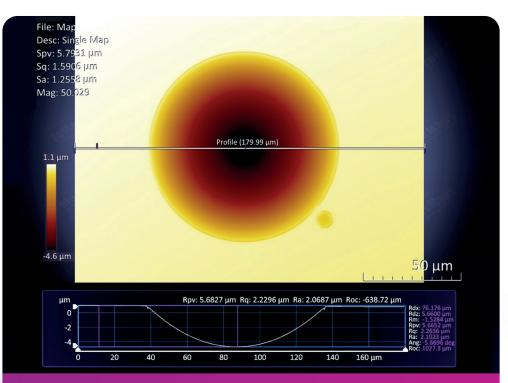
Surface profiling of prototype cavity mirrors at the University of Southampton. [James Gates]
