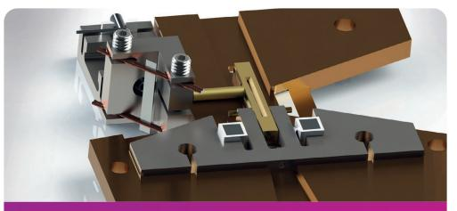
Combined chip trap and optical cavity system under construction at Sussex University. [Matthias Keller]
